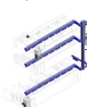
③ NW Laboratory Supply Air Stack - DOAS
